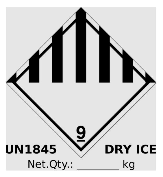
Marking of dangerous goods for transport on dry ice. Print, cut out and stick on the box if you are sending samples on dry ice.
